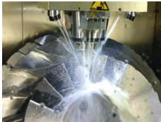
Machining of Impeller for Ammonia Compressor Unit on Germany Hermle 5-axis Machining Center
