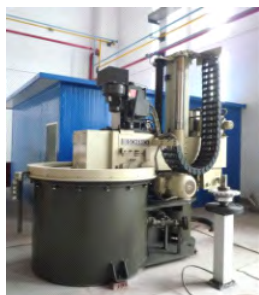
Impeller is doing on dynamic balancing test on Schenck Dynamic Balancing Machine (Germany)
