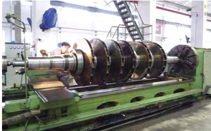
Machining of Six-stage Compressor Rotor in the workshop
