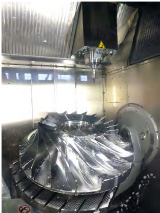
Machining of Impeller for Ammonia Compressor Unit on Germany Hermle 5-axis Machining Center
