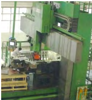
Machining of Cylinder of Compressor on the CNC Dragon Milling and Boring Machine Center
